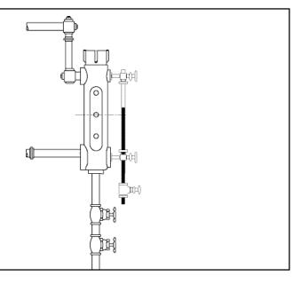
When the water level rises to the level of the top probe, the pump relay will be de-activated. Depending on the application, this will either turn off the pump or close a valve.
