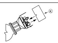
c. Following the appropriate wiring diagram (refer to page 7) based on your application requirements, and using BX armored cable or Thinwall electrical metal tubing connector fittings, make electrical connections to the junction box (L).
