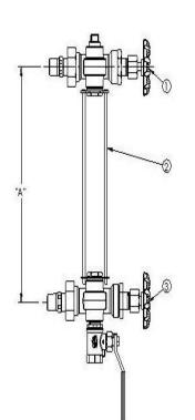
Model 34041 High Pressure Boiler Gauge Fixture Set With Ball Check 250WSP @ 406° F ASME Compliant per B31.1 and Section One, PG 60 Appendix A18 of ASME Boiler Code CRN OCO7137.2C
