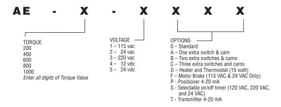
Note: AE will always be the first two characters of the part number, all digits from torque value must be entered into part number (i.e. 400, 1000 etc.) Only use one digit for voltage depiction (i.e. 1-5). For the options listing you may use more than one character, up to three, (i.e. 0, AD or BD etc.)
