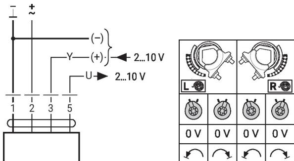
Wiring diagram piggy-back operation (mechanically coupled actuators)
