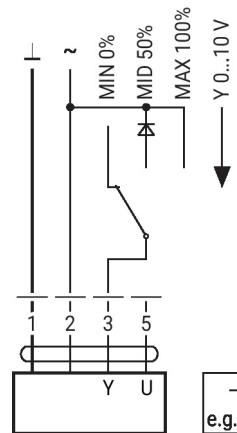
Control remotely 0...100% with positioner SG..
