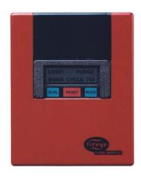
The Flame-Monitor Series provides the proper burner sequencing, ignition and flame monitoring protection on automatically ignited oil, gas and combination fuel burners. On a safety shutdown, the display module will advise the operator that the control is in "Lockout" and indicate the cause as well as the position in the operating sequence that it occurred.
