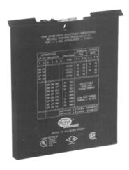
The Fireye EP Programmer Modules are used with the E100 and E110 Flame-Monitor controls. They provide start-up programming, safe-start-check, and flame monitoring supervision. They prove high-fire purge interlock (EP100 series only), low-fire start position and fuel valve end-switch safety checks. A running interlock circuit monitors the limit switches, air flow switches, and fuel pressure switches.
