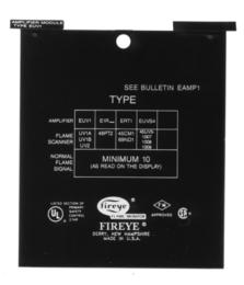
The Fireye Flame Amplifier Modules are used in conjunction with the appropriate flame scanner to provide flame scanning capability in the FLAME-MONITOR system. Fireye offers ultraviolet amplifiers (EUV1), self-check ultraviolet amplifiers (EUVS4), flame rectification amplifiers for use with flame rods and photocells (ERT1), and auto-check infrared amplifiers: E1R1 (standard model), E1R2 (high sensitivity - consult factory before use), and E1R3 (for solid fuels).
