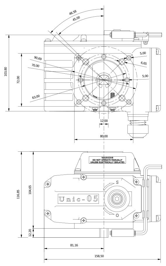
All dimension in millimetres: 1 inch = 25.4 mm
