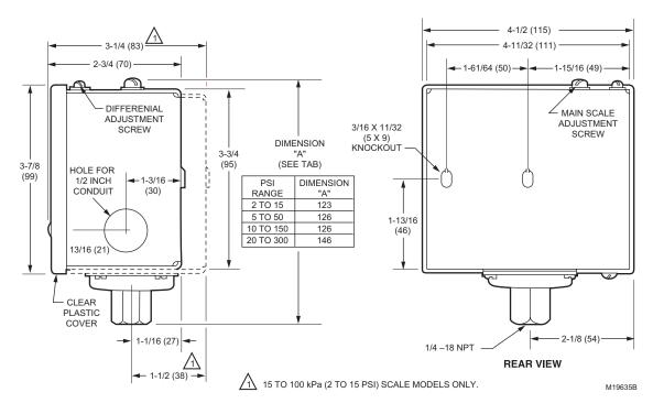
Fig. 1. L404F,T,V approximate dimensions in inches (millimeters in parentheses).
