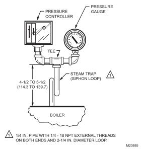
Fig. 2. Steam trap mounting.
