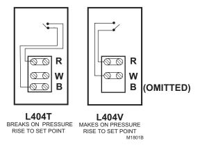
Fig. 8. L404T,V terminal blocks and internal schematics.
