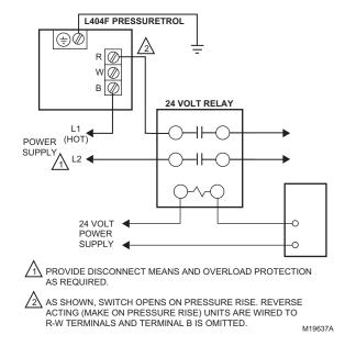
Fig. 6. L404F in low voltage relay circuit.
