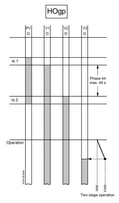
Circulation from Phase 44, max. 45 s as soon as direct heavy oil start = ON in Phase 44: → Phase change in Phase 40 Direct heavy oil start = OFF at the end of Phase 44 → Repetition (max. 3 times in total)
