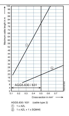
CAN bus connection between power transformer and AZL5... display and operating unit
