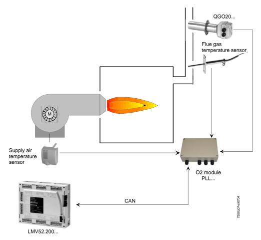
O2 trim control O2 trim controller / O2 monitor The O2 trim controller or O2 monitor can be deactivated or activated in various operating modes by setting a parameter.
