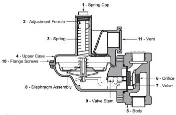
The Model 496 is a general purpose gas pressure regulator for natural gas, air, CO<sub>2</sub>, propane, butane, nitrogen, and other gases. It can be used for gas service to homes, commercial establishments and small industries as well as burners, unit heaters, boilers, and other equipment. All regulators include an internal relief valve.
