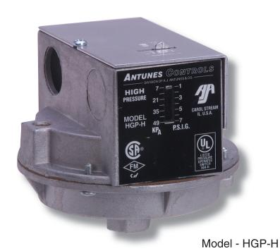
The design and function of the new high pressure gas switches are base on he the same principles of reliability, repeatability and accuracy that has made Antunes Controls existing line of pressure switches so successful. The high pressure gas switch monitors gas pressure and breaks the electrical control circuit when pressure drops below or rises about the desired pre-set point.
