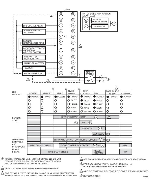
Fig. 2. Wiring subbase and sequence chart for RM7895A,B/EC7895A; RM7896A,B.
