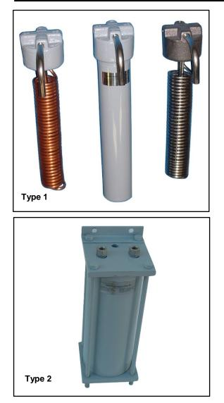
Madden Sample Coolers are miniature heat exchangers designed to reduce high temperature liquid samples to safe, usable temperatures for analysis. They also function as effective coolers for pump seal flush liquid. The counter flow design efficiently cools the tube side liquid.
