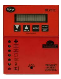
The Fireye® BurnerLogix™ Z System expands on the standard BurnerLogix Y System by combining boiler control functions with the same burner management control found in the Y system. The result is a single compact package that can directly control the boiler's output firing rate based on either input pressure or temperature or both.
